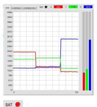
The newly added LED SAT indicates if one of the channels is in saturation. In this case, it lights up red.
